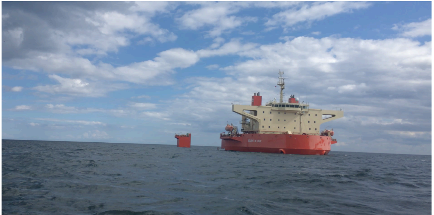
Vessel submerging and waiting at anchorage
