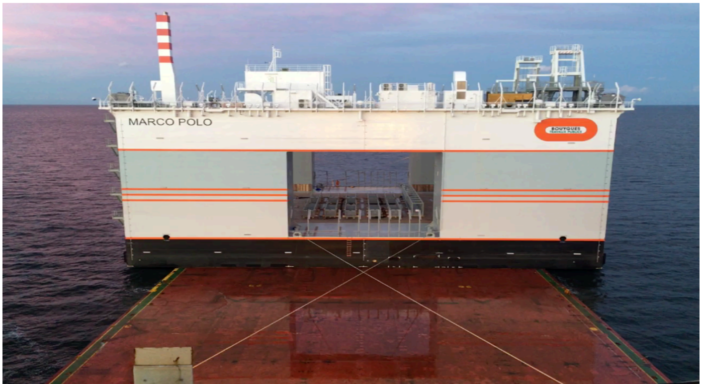
Floating Dock positioned onboard, vessel re-floating.
